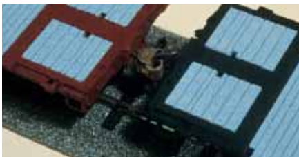
Fig. 5 DELAYED UNCOUPLING. A wide magnet uncouples the cars, then the cars are separated and brought together again with the couplers offset as shown so a car can be shoved and left at a distant location.
