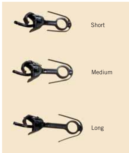
Fig. 2 SHANK LENGTHS. Three shank lengths accommodate different coupler box locations.
