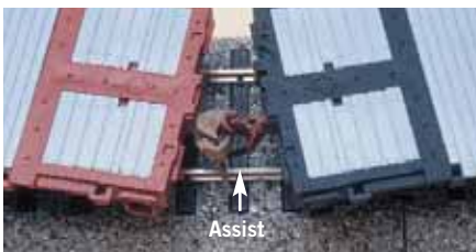
Fig. 6 BAD ANGLE. A bad gathering angle forces different brands of couplers off center toward the outside of a curve so they cannot couple. A manual assist toward the center lets the knuckles open and couple properly.
